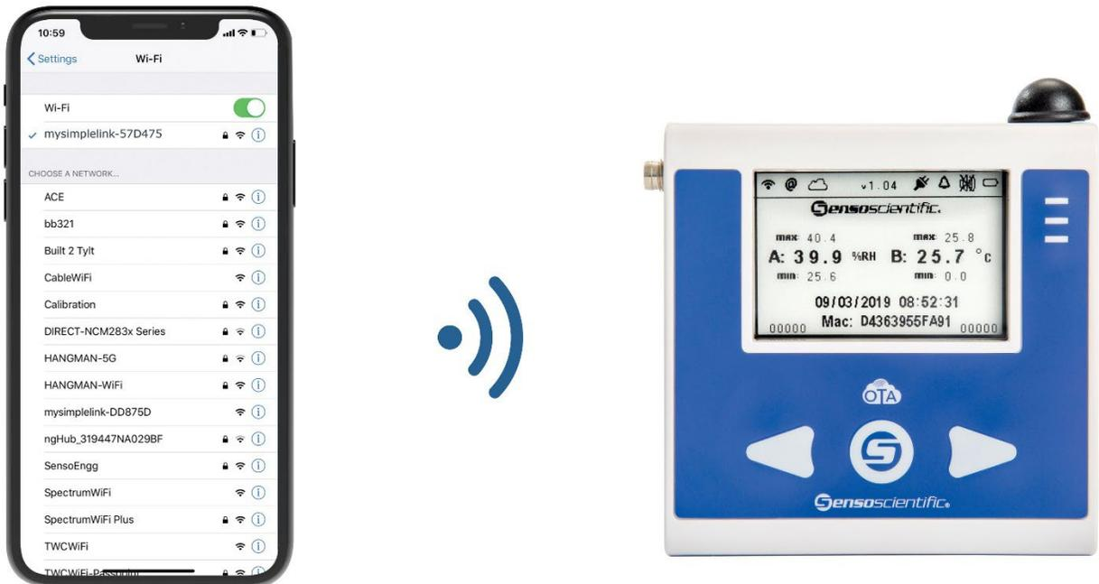
Figure V-3: Connect Wi-Fi enabled device to OTA Node
